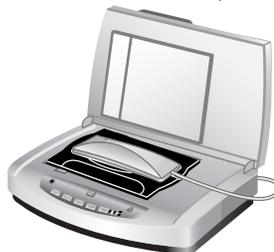
**Place the TMA light source on the positioning plate**
