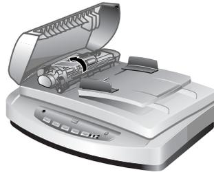
**Lift the green tab to expose the feed rollers**
