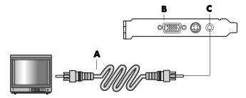
If your TV has a composite video jack and your PC has only an S-video jack, connect a composite video cable to the Video In jack on the TV and to an S-video adapter cable. Connect the S-video adapter cable to the S-video jack on the back of the PC.
