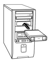
This special drive bay includes an internal USB port and power cable that connect to the drive when it is inserted.
