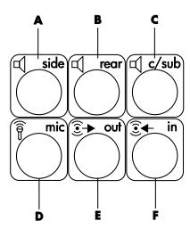
The previous figure shows the six audio connectors arranged on the back of the PC: the four connectors used for eight-channel audio and the connectors for the microphone (**D**, mic) and the audio line in (**F**, in).
