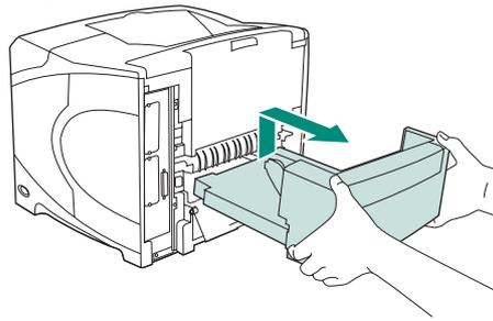
**To remove the duplexer:** Turn the printer so that the rear cover faces you. Lift up and pull out to remove the duplexer.
