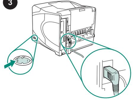
Turn the printer power off. Make sure you are using the right-angle power plug that came with the printer.
