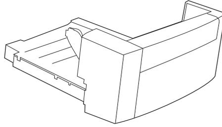
Remove the orange tape and all packing material from the duplexer.
