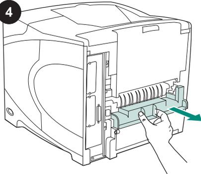
Remove the duplex-slot cover from the back of the printer.
