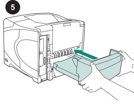
Using both hands, insert the duplexer all the way into the slot.
