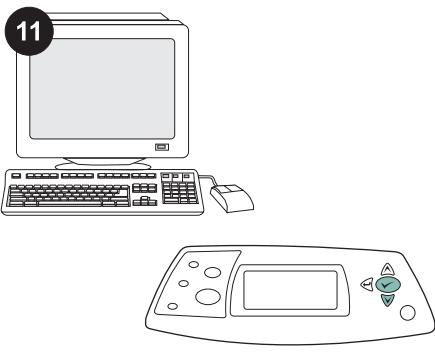
Select duplex or two-sided printing from your program. If neither of these options is available in the program, use the printer control panel menus to turn on duplexing. For more information, see the use guide on the CD-ROM that came with the printer.
