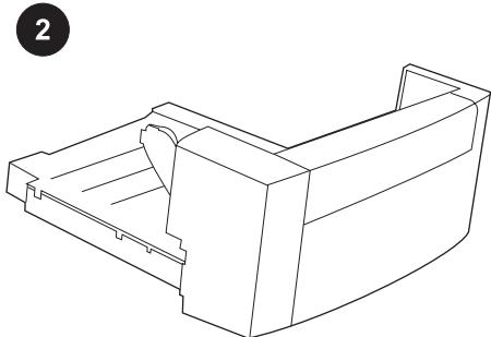
Remove the orange tape and all packing material from the duplexer.
