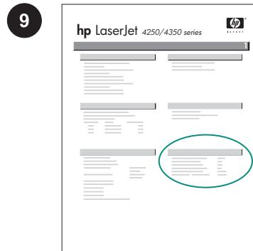
Make sure that the configuration page lists the duplexer as an installed accessory. If the duplexer is not listed, see the use guide on the CD-ROM that came with the printer.
