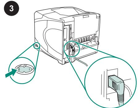
Turn the printer power off. Make sure you are using the right-angle power plug that came with the printer.
