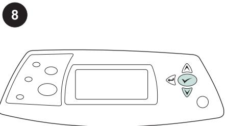
To verify that installation is complete, print a configuration page from the control panel. Press **✓** to open the printer menus. Press **▼** to select **INFORMATION**, and then press **✓**. Press **▼** to select **PRINT CONFIGURATION**, and then press **✓**.
