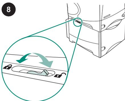
Move the tray-lock lever (located along the top-left side of the tray) into the locked position for each installed tray.
