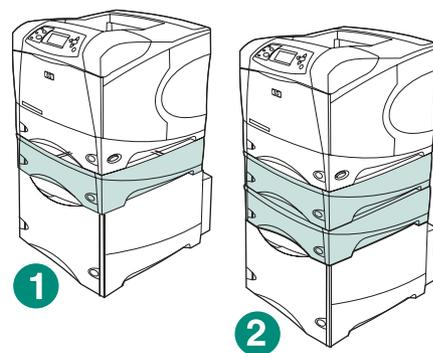
For the HP LaserJet 4200/4300 series, one optional 500-sheet feeder can be installed on top of the optional 1,500-sheet feeder (callout 1).
