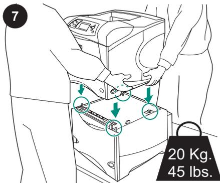
Position the 1,500-sheet feeder where the printer will be located. Using the handles on the sides of the printer, lift the printer onto the 1500-sheet feeder. Align the holes in the base of the printer with the mounting pins on the 1500-sheet feeder.
