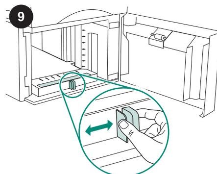
Open the door of the 1500-sheet feeder. Pinch the levers at the front of the feeder and slide them to the letter (LTR), legal (LGL), A4 paper size setting.
