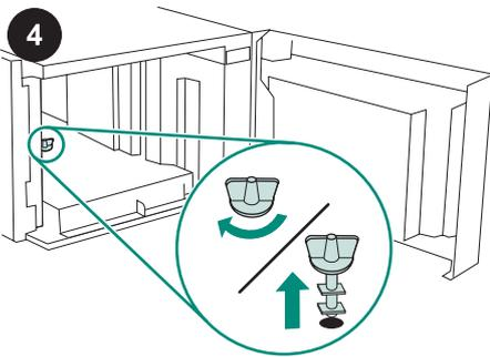
**CAUTION** The 1,500-sheet feeder tray lock *must* be removed before operating the feeder. Turn the feeder tray lock clockwise, and then pull the lock up and out of the feeder.
