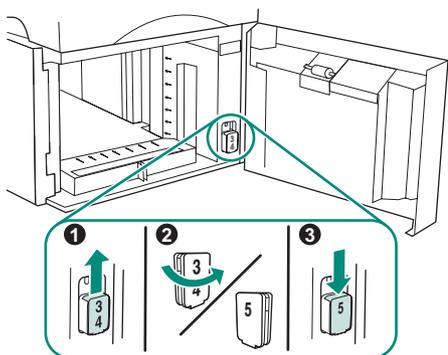
**HP LaserJet 4250/4350 only:** If the 1,500-sheet feeder is tray 5, open the feeder door, remove the tray-number-indicator block (callout 1), turn it around (callout 2), and reinstall it so that the number 5 will show through the slot in the door (callout 3). If the feeder is any other tray, proceed to the next step.
