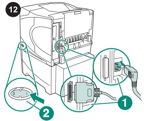
Connect the cables to the rear of the printer (callout 1). Turn the printer power on (callout 2).
