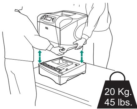
To prevent possible injury or damage to the printer, separate the printer from any currently installed optional feeders before lifting the printer (two people should lift the printer).
