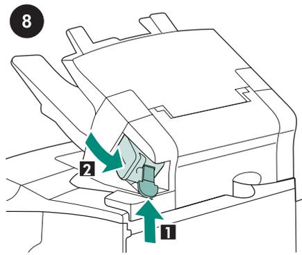
If your device is a stapler/stacker, make sure that the staple cartridge (callout 1) is installed, and that the stapler unit is snapped into the closed position (callout 2).
