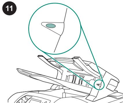
Make sure that the light on the front of the stacker or stapler/stacker is solid green. If the light is amber, flashing, or off, see "Understanding the accessory lights for the stacker and stapler/stacker" in the use guide on the CD-ROM that came with the printer.
