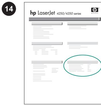
Make sure that the configuration page lists the stacker or stapler/stacker as an installed accessory. If the stacker or stapler/stacker is not listed on the configuration page, see the use guide on the CD-ROM that came with the printer.
