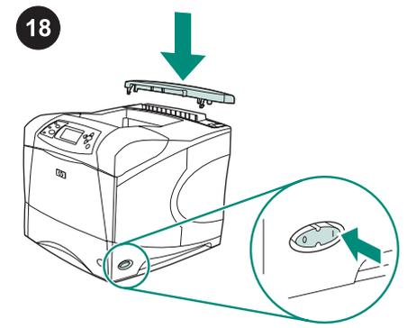
Reinstall the accessory cover. Turn the printer power on.
