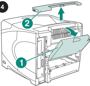
Open the rear output bin (callout 1). Remove the accessory cover located at the top-rear of the printer (callout 2). Close the rear output bin.
