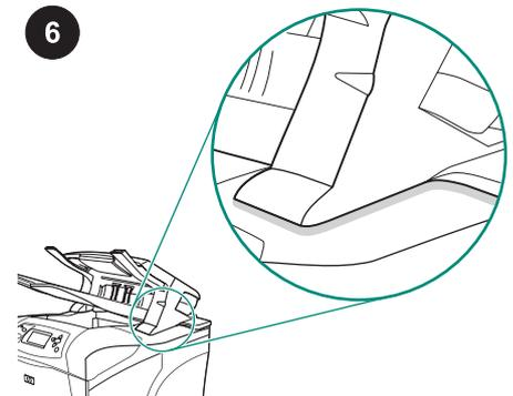
Make sure that the stacker or stapler/stacker is completely seated.
