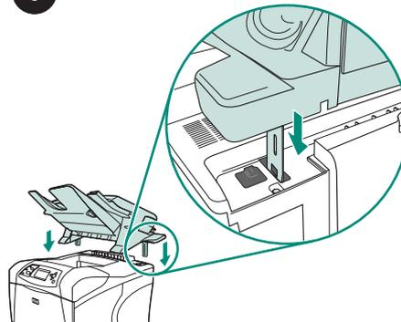
Firmly gripping the stacker or stapler/stacker, insert the metal legs into the slots at the top-rear of the printer.
