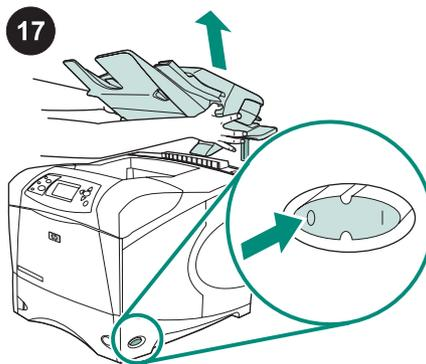
**To remove the stacker or stapler/stacker.** Turn the printer power off. Lift the stacker or stapler/stacker upward until the metal legs are removed from the slots in the printer.
