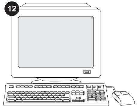
To take advantage of all the stacker or stapler/stacker functions, the printer driver on the printer's host computer must be configured to recognize the stapler/stacker or stacker. For Windows®, go to the printer Properties window. On the **Device Settings** tab, select the check box for the stacker or stapler/stacker.
