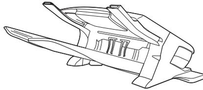
Remove the orange packing tape and all packing material from the stacker or stapler/stacker.
