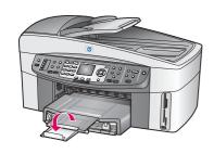
To prevent paper from flying out of the output tray, pull and then flip the paper tray extender out.
