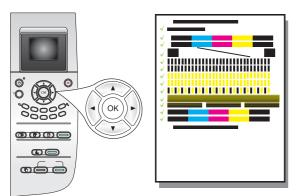
**a** Press **OK** at each of the prompts on the control panel to start print cartridge alignment.
