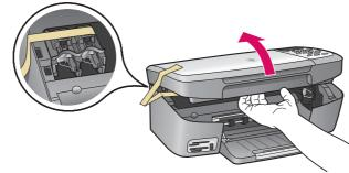
Lift the access door and remove tape inside the left side of the device.
