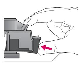
The device must be **On** before you can insert the print cartridges.
