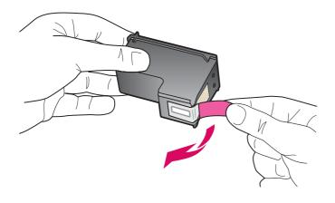
Pull the pink tab to remove the tape from **both** print cartridges.
