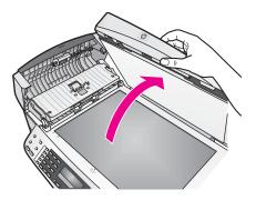
3 Lift the automatic document feeder mechanism.
