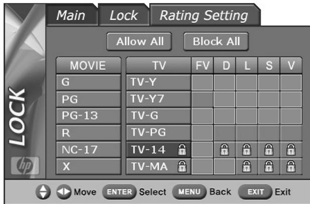
6 Use the arrow buttons on the remote control to move your cursor into the block you would like to lock. Press the Select button to lock the rating.
