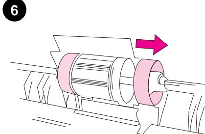
Slide the idler roller to the right to separate it from the pickup roller.
