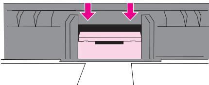
Snap both sides of the separation pad firmly into place until they click. **CAUTION:** If the pad is not straight, or if space exists between the pad and the base, make sure that the tabs on the pad are toward the front of the printer.
