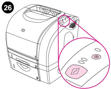
When the green Ready light is on, press **Go** to print a Demo page, which verifies that the printer works and that installation is complete.
