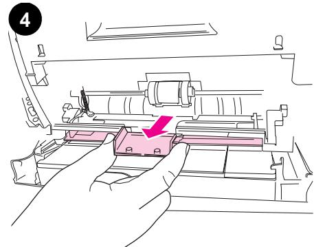
Grasp both sides of the center tab and pull the cover out of the printer.
