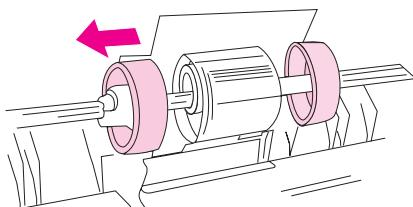
Slide the idler roller to the left to separate it from the pickup roller.
