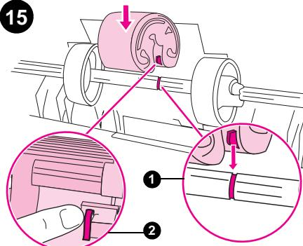
Hold down the new separation pad. (1) Position the new pickup roller so that the button is on the right side, and the open side of the roller faces down. (2) Make sure that the small ridge on the open side of the roller aligns with the groove in the shaft.
