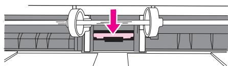
Locate the separation pad beneath the area of the shaft from which the pickup roller was removed.
