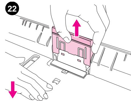
Pull the separation pad up and out of the tray.
