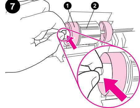
Squeeze the tab on the (1) idler roller that is located on the left side of the (2) pickup roller. If the tab is not visible, rotate the idler roller so that the tab is toward the front of the printer.
