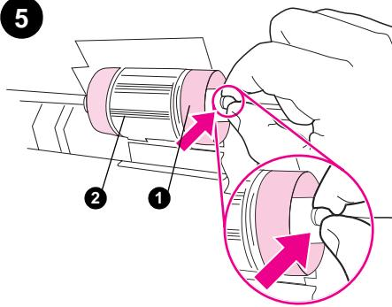
Squeeze the tab on the (1) idler roller that is located on the right side of the (2) pickup roller. If the tab is not visible, rotate the idler roller so that the tab is toward the front of the printer.
