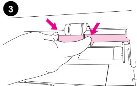
Find the faceplate cover that is located beneath the pickup roller in tray 1.
