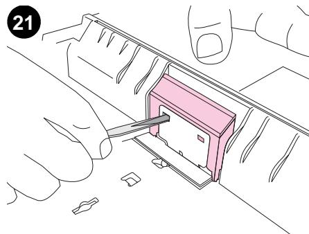
Press the large metal plate at the bottom of the tray down. Insert a flatblade screwdriver in the slots on each side of the base and push the tabs out of the slots. **Note:** In a 250-sheet tray, the plate locks down; in a 500-sheet tray, you have to hold the plate down manually.
