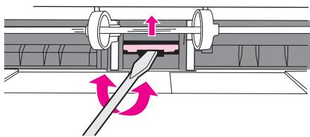
Insert a flatblade screwdriver into the slot under the separation pad. Pry the pad up from the spring-loaded base by twisting the screwdriver until the tabs are separated from the printer.
