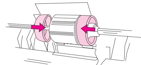
Slide the left and right idler rollers inward, against the pickup roller, until the idler rollers click into place.
