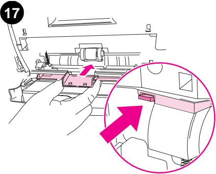
Hold the faceplate cover as shown in the illustration, and align the cover with the rails on the inside of the printer.
