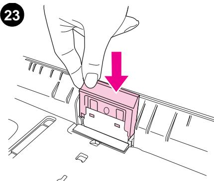
Use one hand to position the new separation pad above the empty base. Align the grooves on the sides of the pad with the sides of the base, and then slide the pad down until the tabs snap into the slots on the base.
