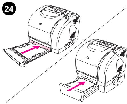
Reload any print media that you removed, and then slide the tray into the printer.
