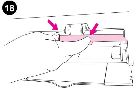
Grasp both sides of the center tab and insert the cover into the printer until the cover clicks into place. Close tray 1.
