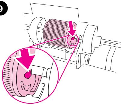
Press and hold the button that is located on the right side of the pickup roller. Slide the pickup roller slightly to the right, and then pull it off of the shaft. **CAUTION:** To prevent the shaft retaining pin from falling out, do not move the remaining hub that is located to the left of the pickup roller.
