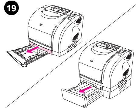
**Replace the separation pad in tray 2 or in optional tray 3.** Remove the tray from the printer and place it on a flat surface. Remove any print media from the tray.
