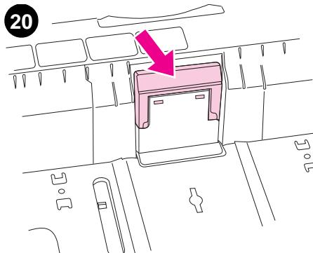
Locate the separation pad in the base at the inside-front edge of the tray.
