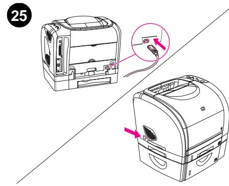
Reconnect the power cable. Turn the printer on.
