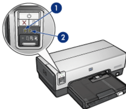
1 . The left status light represents the tri-color print cartridge.
