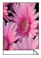
If the border appears above the tear-of tab, then align the print cartridges.
