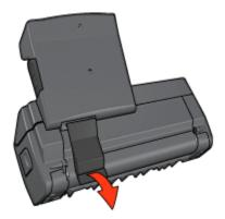
5. Tilt the Small Paper Tray forward and open the lower door of the accessory.
