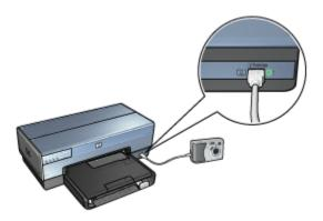
After you successfully connect the camera to the printer, you can print your photos. Be sure the size of the paper loaded in the printer matches the setting on your camera. Refer to the documentation that came with your camera for detailed information on printing from the camera.
