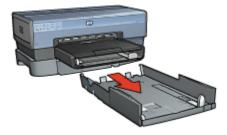
2. Slide the paper-width guide until the arrow is even with the correct setting.
