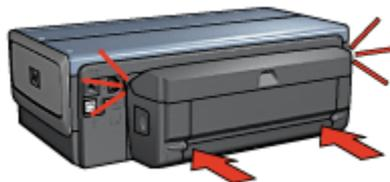
Note: Do not press the buttons on either side of the duplexer when installing it in the printer. Use the buttons only when removing the duplexer from the printer.
