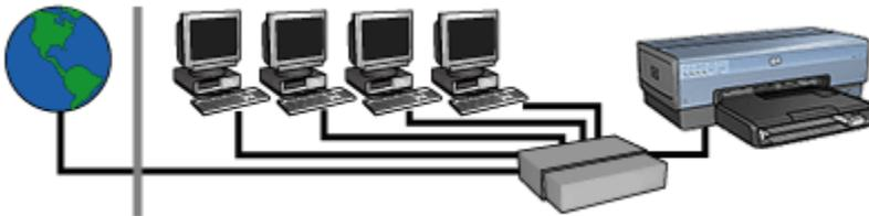
This example looks similar to the first example. However, in this example, the network devices are connected to a [hub](#), rather than a [router](#). The hub is directly connected to the Internet.
