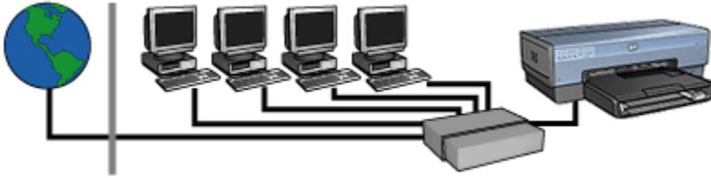
In this example, a [router](#) manages the network connections and acts as a [gateway](#) between the network and the Internet.
