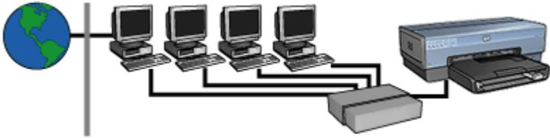
In this example, the network devices are connected to a [hub](#). A computer on the network acts as the [gateway](#) between the network and the Internet. The gateway computer uses [Windows Internet Connection Sharing \(ICS\)](#) to manage the network connections and provide Internet access to the other devices.
