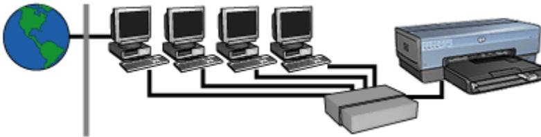
In this example, the network devices are connected to a [hub](#). A computer on the network acts as the [gateway](#) between the network and the Internet. The gateway computer uses [Windows Internet Connection Sharing \(ICS\)](#) to manage the network connections and provide Internet access to the other devices.
