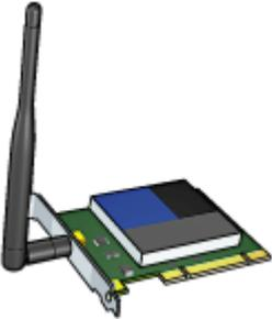
An ISA or PCI card, which is a green printed circuit board with a blue and black component on top and a long metal edge connector at the bottom, used for desktop computers.     | ISA or PCI card that can be used with a desktop computer.                  |
