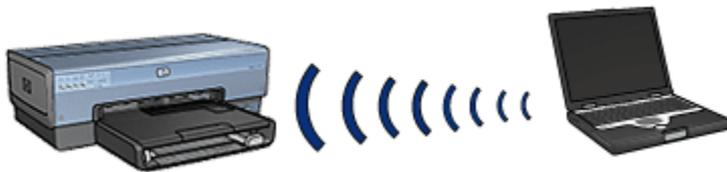
Ad hoc networks are typically small and simple. Performance on these types of networks can degrade if more than six devices are on the network.
