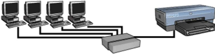
In this example, the network devices are connected to a [hub](#). Devices use [AutoIP](#) to obtain IP addresses.
