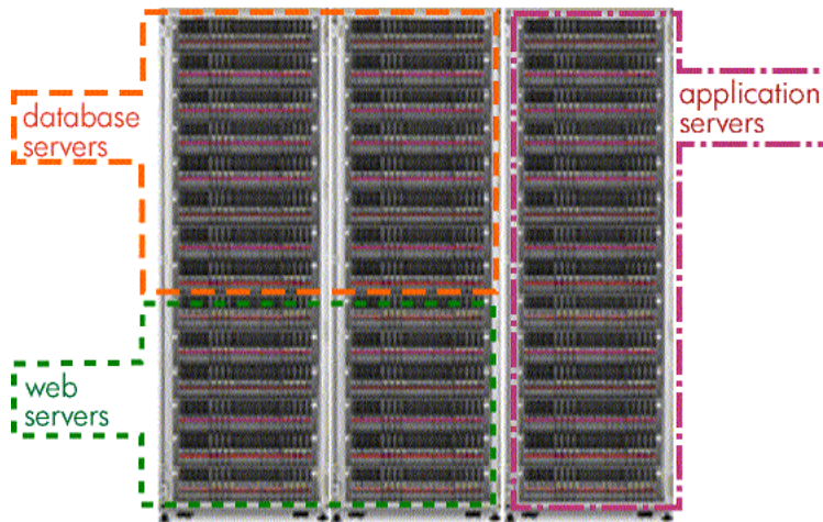
Figure 5. Fabrics will enable data centers to achieve higher CPU densities and better computing resource efficiency with blade servers.
