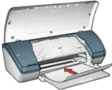
5. Carefully push the transparencies into the printer until they stop so that none of the adhesive strips catch on one another.
