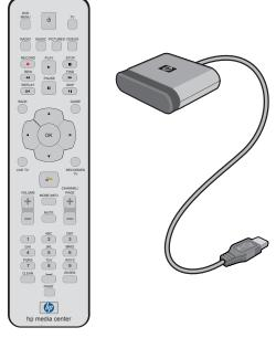
Use the remote control at a maximum distance of 26 feet (8 meters) from the remote sensor and at a maximum of 22.5 degrees (45 degrees total) from the center of the remote sensor.
