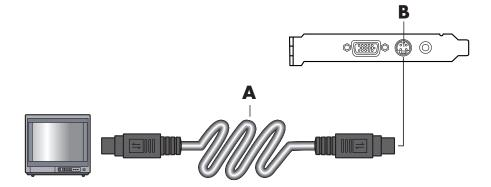
4 If your TV has a composite video jack and your PC has a composite video jack, connect a composite video cable (A) to the Video In jack on the TV to the composite Video Out jack (C) on the back of the PC.
