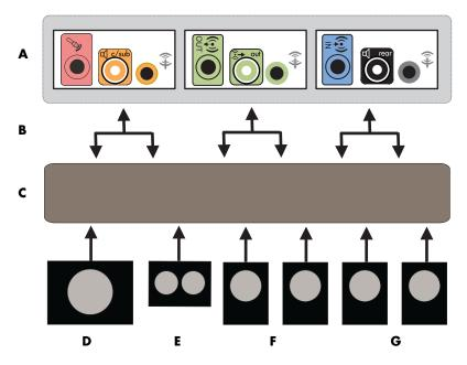
PC to 5.1 multichannel audio system connection
