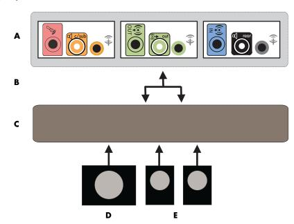
PC to 2.1 multichannel audio system connection
