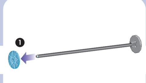
Remove the blue-colored stop (A) from the left-hand end of the spindle. Keep the spindle horizontal.
