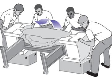
Using four people and the hand holds on the rear of the printer body, carefully lift the printer into an upright position.
