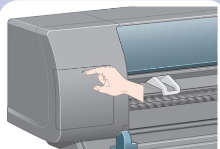
Find the ink cartridge door, which is on the left side of the printer.
