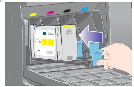
Push the ink cartridge drawer back into the printer until it locks into position.
