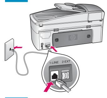
Connect one end of the supplied phone cord to the phone port on the left **(1-LINE)** and the other to a wall jack.
