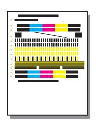
**a** Press **OK** at each of the prompts on the control panel to start print cartridge alignment.
