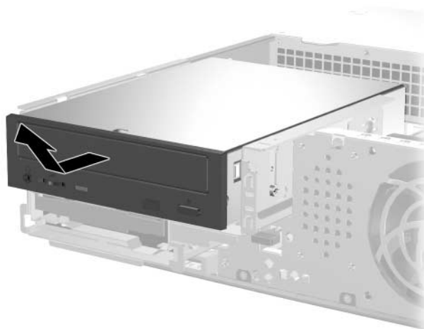
Removing the Optical Drive
