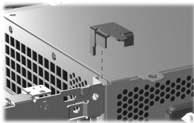
Installing the Security Clip
