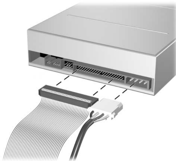
Disconnecting the Power and Data Cables
