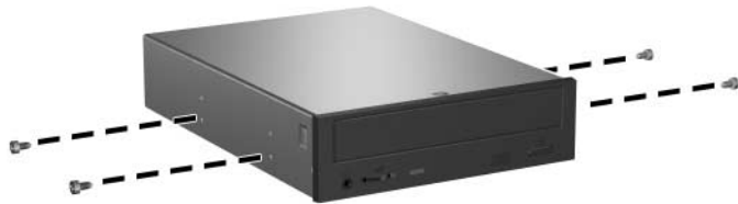
Installing Guide Screws in the Optical Drive
