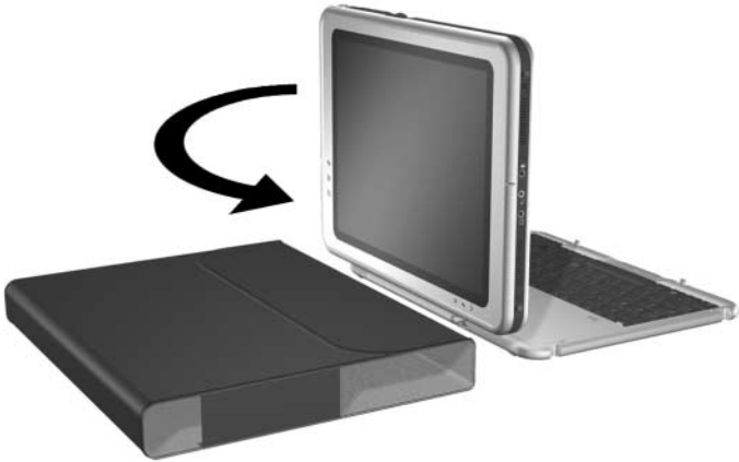
Positioning the assembly for the battery pack insertion
