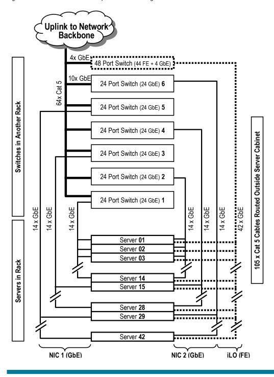
Figure 9. Maximum Performance Density Ethernet Cable Diagram
