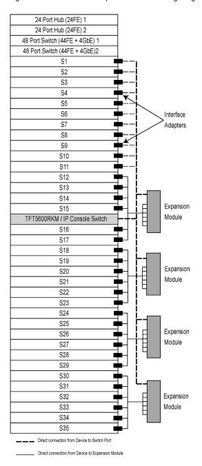
Figure 12. Maximum Flexibility Ethernet Cable Diagram
