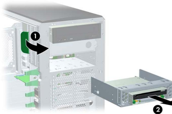
4. Remove the diskette drive by removing the two M3 screws ❶ in the rear-most holes and sliding the diskette drive ❷ from the bracket.
