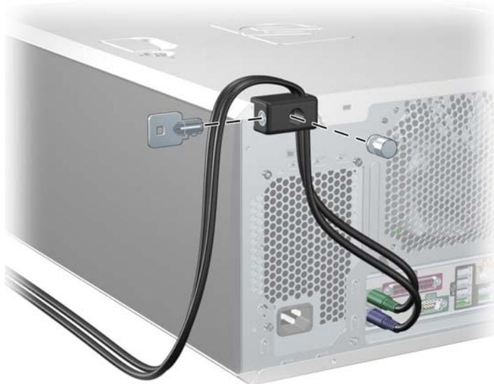
2. Remove the screw attaching the lock to the chassis.
