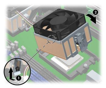
6. On the opposite side, push down on the CPU heatsink to clip the other metal latch over the plastic frame. If necessary, use a flat-bladed screwdriver to snap the latch over the hook on the plastic frame.
