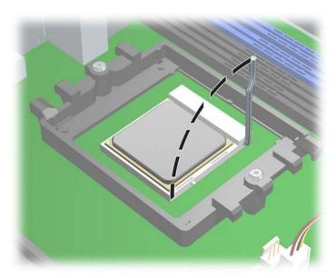
3. Pull the processor straight out of the socket.
