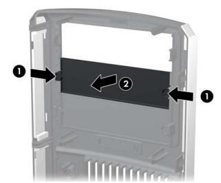
To replace the bezel blank, push in on the tabs and push the bezel blank into the bezel.
