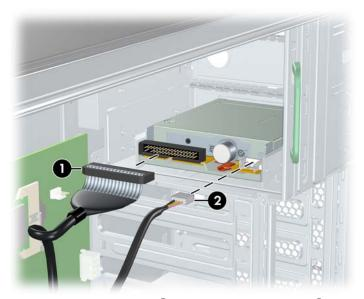
3. While lifting the green drivelock release tab **1**, slide the drive forward **2** out of the chassis.
