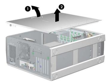
To replace the access panel, slide the cover back on until it snaps into place.
