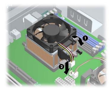
9. Double check and be sure the latch lever is snapped to the plastic frame correctly. The lever must attach to the plastic frame exactly as shown in the following illustration.
