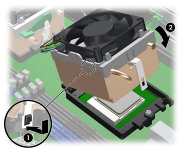
6. On the opposite side, clip the metal latch over the plastic frame.
