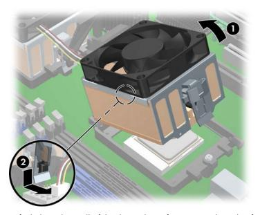
10. Use alcohol and a soft cloth to clean all of the thermal interface material residue from the CPU heatsink and processor.
