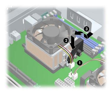
6. On the opposite side where the lever is placed, press down on the metal clamp **1** (illustration below) until the tab releases from the processor retention frame.
