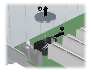
To replace the battery, slide the battery back in until it snaps back into place.
