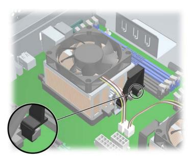
10. Lower the CPU airflow duct over the CPU heatsinks until it snaps into place.
