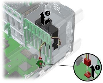
4. Remove the fan from the fan housing by applying outward pressure on the fan housing while pushing the fan out of the housing.
