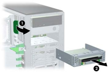
4. Remove the diskette drive by removing the two M3 screws 10 in the rearmost holes and sliding the diskette drive **2** from the bracket.
