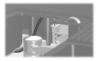
Disconnecting the Fan Cable, Compaq Presario R4000 Models
