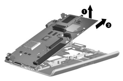
Removing the System Board
