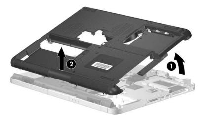
Removing the Base Enclosure, Compaq Presario R4000 Models
