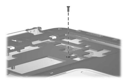
Removing the Thermal Frame Screw
