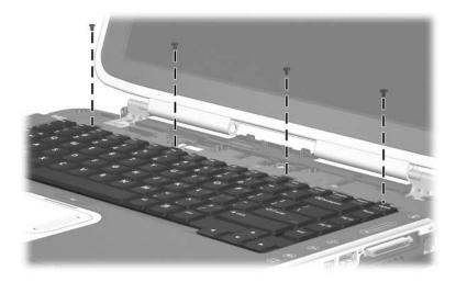
Removing the Keyboard Screws
