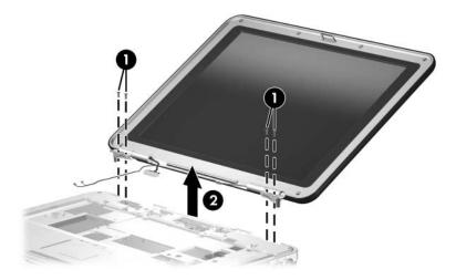
Removing the Display Assembly, Compaq Presario R4000 Models
