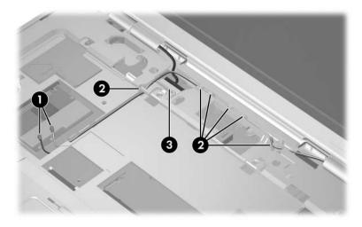
Removing the Display and Wireless Antenna Cables, Compaq Presario R4000 Models
