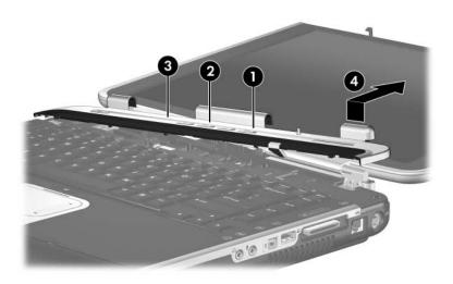
Removing the Keyboard Cover, HP Pavilion zv6000 Models
