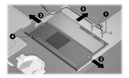
Removing a Mini PCI Communications Card
