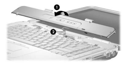
Removing the Keyboard Cover, Compaq Presario R4000 Models
