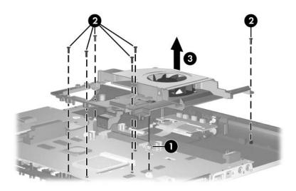
Removing the Thermal Frame
