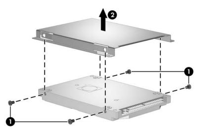
Removing the Hard Drive Frame
