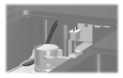
Disconnecting the Fan Cable, HP Pavilion zv6000 Models
