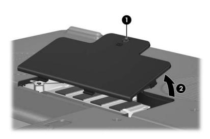
Removing the Memory Module Compartment Cover
