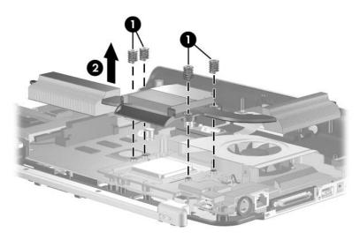
Removing the Thermal Module
