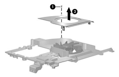
Removing the Fan Shield
