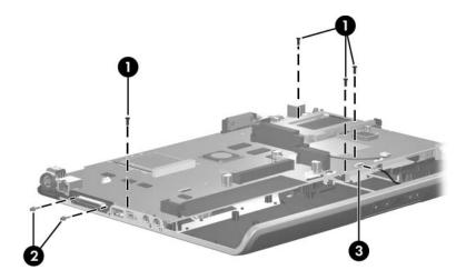
Removing the System Board Screws
