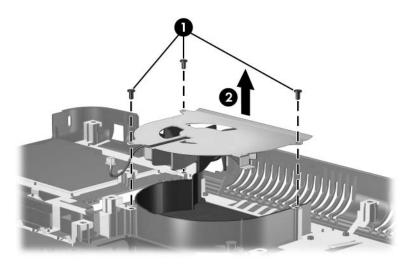
Removing the Fan Assembly
