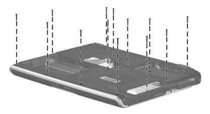
Removing the Base Enclosure Screws, Part 1, HP Pavilion zv6000 Models 4. Remove the four PM2.0×7.0 screws that secure the base enclosure to the notebook.
