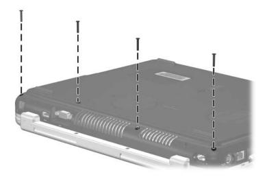
Removing the Keyboard Cover Screws
