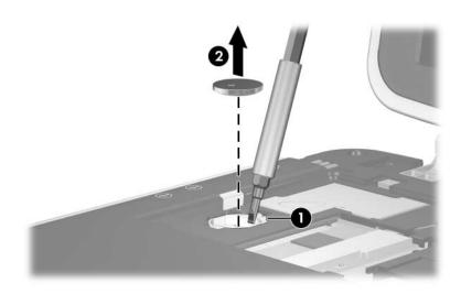
Removing the RTC Battery
