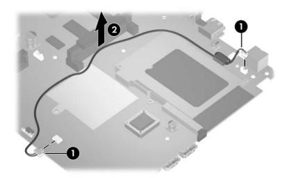
Removing the RJ-11 Modem Cable
