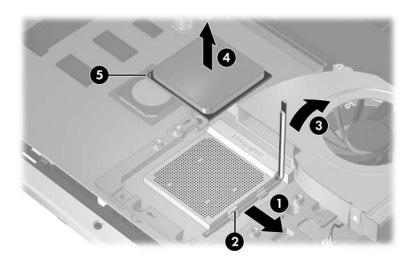
Removing the Processor
