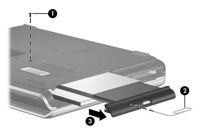
Removing the Optical Drive
