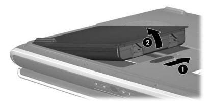
Removing the Battery Pack
