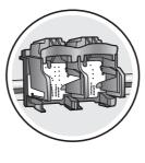
Lower the access door until it stops. Make sure the print carriage moves to the center.
