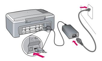
**Important:** Do not connect the USB cable until instructed later in this guide.
