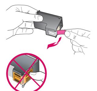
Pull the pink tab to remove the tape from **both** print cartridges.
