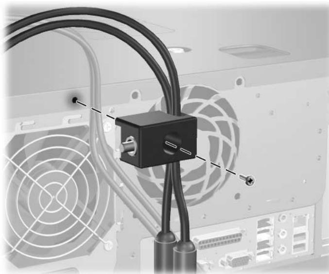
4. Insert the plug end of the security cable into the lock ❶ and push the button in ❷ to engage the lock. Use the key provided to disengage the lock.
