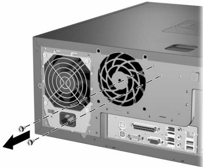
*Removing the Smart Cover Lock Screws*
