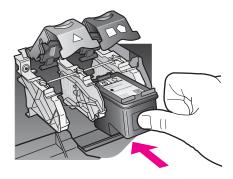
Press down on the latch until it stops. Make sure the latch catches below the bottom tabs.
