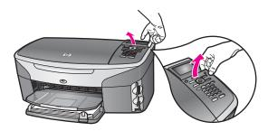
Tip You can also use a thin, flat object, such as a credit card, to lift the control panel overlay. Gently slide the credit card at a slight angle, about 45 degrees, between the color graphics display and the control panel overlay. Apply slight downward pressure to lift the control panel overlay.
