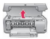
Squeeze the gray tab below an ink cartridge slot to release the gray latch inside the printer, then lift the latch.
