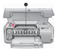
1 Open the paper jam door to clear paper jams in the middle of the printer.
