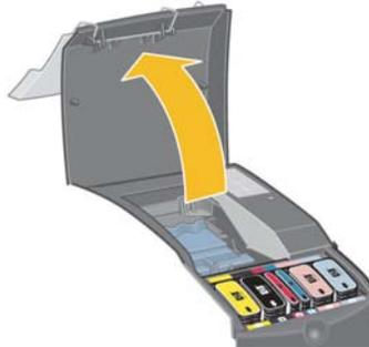
4. Remove the failed printhead by lifting the small handle at the top front and using it to pull the printhead vertically up and out of the printer.
