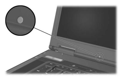
You can turn on and off the ambient light sensor using the Quick Launch Buttons software:
