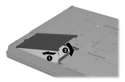
4. Tighten the screws on the hard drive bay cover.
