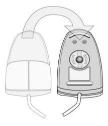
2. Remove the ball from your mouse and clean it with an antistatic wipe or a lint-free cotton cloth.
