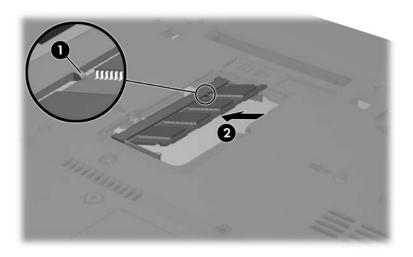
c. Press the module downward until the retention clips snap into place.
