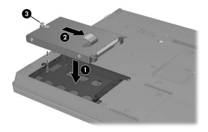
3. Align the tabs on the hard drive cover with the slots on the notebook • and press the hard drive cover down until it fits into place •.
