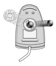
3. Spray the inside of the mouse with compressed air or clean it with a noncotton swab to remove loose debris and dust.
