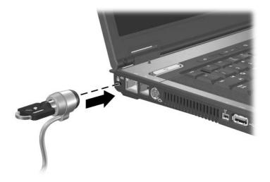
3. Turn the key counterclockwise **①**, remove the key **②**, and store the key in a safe location.
