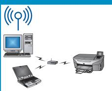
Use this connection type if you want a wireless (802.11 b or g) connection between the device and your network.
