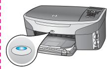
If you are not using a wireless network and want to turn off the blue light, press **Setup**, **8**, **5**, and then **2**.
