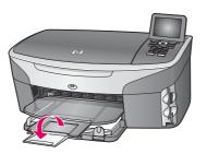
To prevent paper from flying out of the output tray, pull, and then flip the paper tray extender out.
