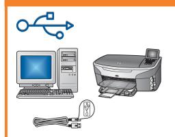
Use this connection type if you want to connect the device directly to one computer. (Do not connect until the software instructs you to.)
