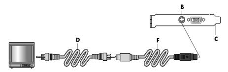
**NOTE:** The S-video adapter cable is only needed if there is no composite video jack on the back of the PC.
