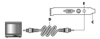
If your TV has a composite video jack and your PC has only an S-video jack, connect a composite video cable to the Video In jack on the TV and to an S-video adapter cable. Connect the S-video adapter cable to the S-video jack on the back of the PC.
