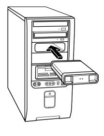
This special drive bay includes an internal USB port and power cable that connect to the drive when it is inserted.
