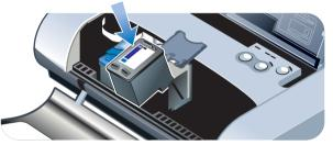
5 Close the print cartridge latch. If the cartridge is inserted correctly, closing the latch gently pushes the cartridge into its socket. Press the latch to make sure it is seated flat on the cartridge.
