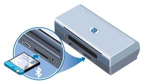
5 Press the Resume button to print the images. The printer will automatically recognize the DPOF file on the CF card and print the images according to the specifications you set in the file.
