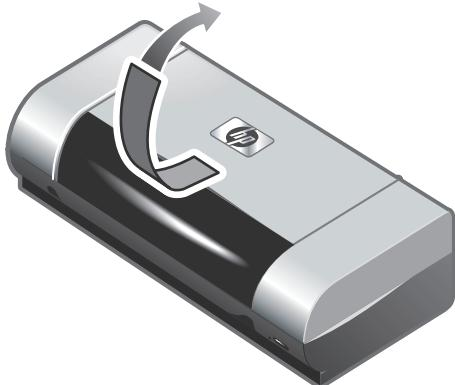
**Step 2: Remove the packing tape.**
