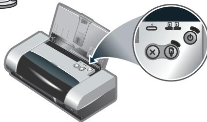
**Note:** Use only the C8222A battery with the printer. Fully charge the battery before using (approximately 1 hour and 30 minutes). When the battery is charging, the battery charge LED is green. If the LED is red while charging, the battery might be faulty and need to be replaced.
