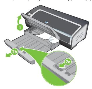
5 Open the top cover. The print cartridge carriage should return to the right side of the printer. If the carriage does not return to the right side, turn off the printer, and then move the carriage to the right. Pull any jammed paper towards you.
