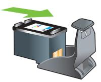
2 To remove the print cartridge from the protector, press down and back on the tab inside the protector to release the print cartridge, and then remove the print cartridge.
