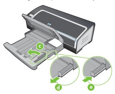
f Reload the desired media into the output tray (see <u>Loading media in the input tray</u>).
