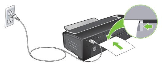
3 Press the Resume button to proceed with printing. If you are printing more than one page, press the Resume button after inserting each sheet of paper.
