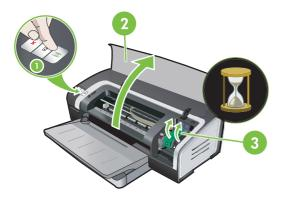
2 If you are replacing a print cartridge, grasp the installed print cartridge and slide it out of its cradle. To ensure you are placing the new print cartridge into the correct position, verify the symbols on the latch match the symbols on the new cartridge.
