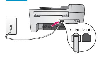
Connect one end of the supplied phone cord to the phone port on the left (1-LINE) and the other to a wall jack.
