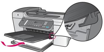
d Attach the top (output) tray. Make sure you hook the top edge of the tray into the light gray latches, and then lower.
