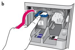
The device must be **On** before you can insert the print cartridges.
