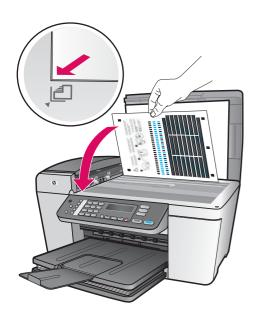
After you insert the cartridges, a message appears that the device is ready for alignment.
