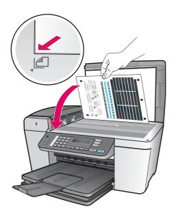
After you insert the cartridges, a message appears that the device is ready for alignment.
