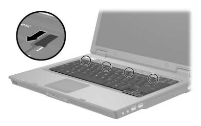
11. Gently lift the top edge of the keyboard and tilt the keyboard over until it rets on the palm rest of the notebook.
