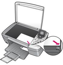
c Place the photo (face down) on the right front corner of the glass. Make sure the long edge of the photo is along the front of the glass. Close the lid.
