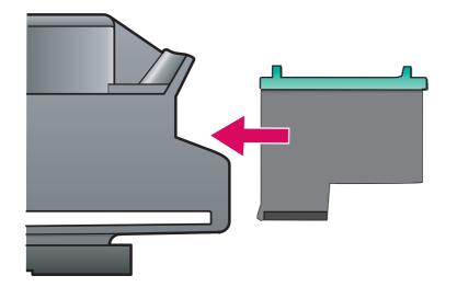
The device must be **On** before you can insert the print cartridges.
