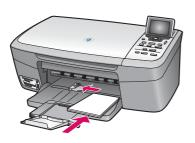
a Remove the plain white paper and load the 4 x 6 in (10x15 cm) photo paper. Place the paper glossy side down. Move the paper adjusters next to the stack of paper.
