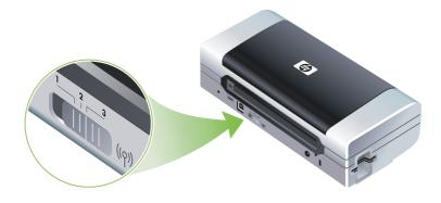
For example, if you configured profile 1 for printing in an infrastructure environment (for example, the office) and configured profile 2 for printing in an ad hoc environment (for example, away from the office or on the road), you only have to move the switch between 1 and 2 to switch between those profiles.
