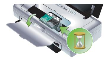
3. Lift the print cartridge latch open and gently remove the print cartridge from its cradle compartment.
