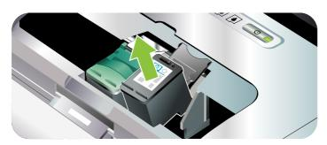
4. Insert the new print cartridge into its cradle compartment at the same angle at which you removed the old print cartridge. Check the number on the latch against the number on the print cartridge to make sure you are inserting the correct print cartridge.
