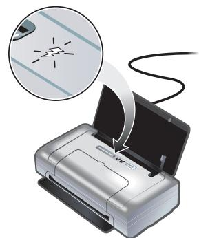
Fully charge the battery before using (approximately 4 hours for the first charge, 2 hours for subsequent charges). When the battery is charging, the battery charging light is green. If the light is red while charging, the battery might be faulty and need to be replaced. See the onscreen user's guide on the Starter CD for instructions on replacing the battery.
