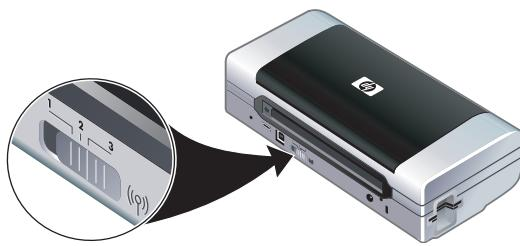
**Note:** Current 802.11 settings will be saved to the current position of the wireless profile switch. The wireless profile switch is used to switch between 802.11 profile settings when changing wireless networks. See "About 802.11 wireless printing" on 25 for information about configuring wireless settings.
