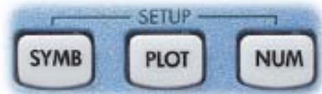
In particular, the **SYMB SETUP** key is only used in one place, which is to choose the data model for bivariate statistics in the Statistics aplet. It is not available in the other aplets and trying to access it will result only in a quick flash of an exclamation mark on the screen to say "You've done something wrong!".
