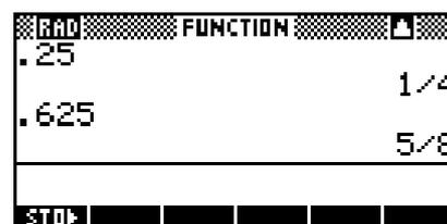
Not understanding the significance of the setting of Fraction can produce some unfortunate effects. For example, at Fraction 2, the value of 123.456 becomes 123, with the 0.456 dropped entirely.
