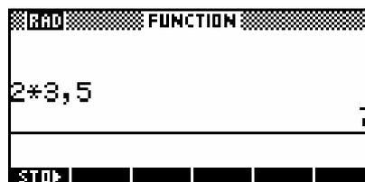
If you opt to use a comma rather than a full stop then any places where a comma would normally be used (such as in lists) will swap to using a full stop. Any functions which might normally have terms separated by a comma will use a full stop instead. For example, **ROUND(3.456,2)** will become **ROUND(3,456.2)**.
