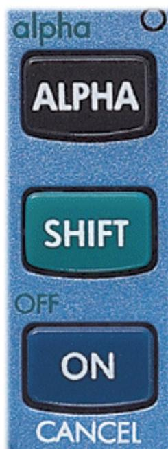
The **SHIFT** key gives you the second function for each key. In the case of the **COS** key, the second function is **ACOS**, sometimes referred to as arc-cos or  $\cos^{-1}$  or inverse cos. Most keys have these second functions that are obtained via the **SHIFT** key.
