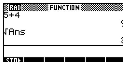
Above the **ENTER** key is the **ANS** key. This can be used to retrieve the final value of the last calculation done. An example of this is shown right.
