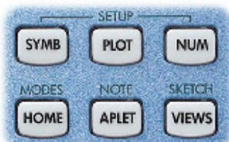
The **APLET** key is used to choose between the various different aplets available. Everything in the calculator revolves around aplets, which you can think of either as miniature programs or as environments within which you can work.
