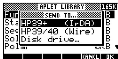
To send an aplet, both calculators should be showing the **APLET** view, with the highlight on the aplet you wish to send. Now press the **SEND** key on the sending calculator and the **RECV** key on the receiving calculator.
