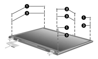
Removing the Display Bezel Screws, HP Pavilion dv4000 Models
