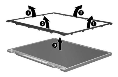
Removing the Display Bezel
