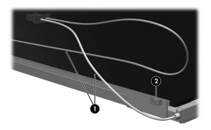
Releasing the Backlight Cables
