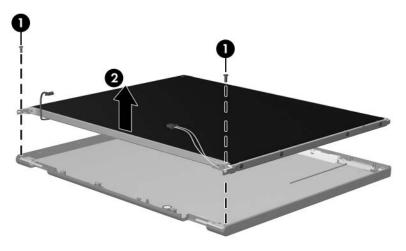
Removing the Display Panel Assembly
