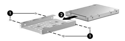
Removing the Hard Drive Frame
