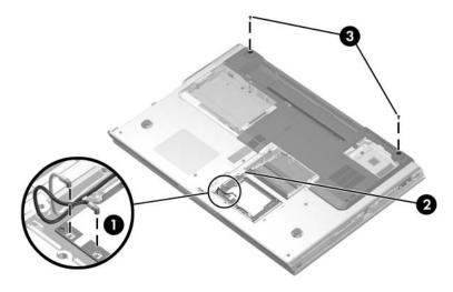
Removing the Display Screws
