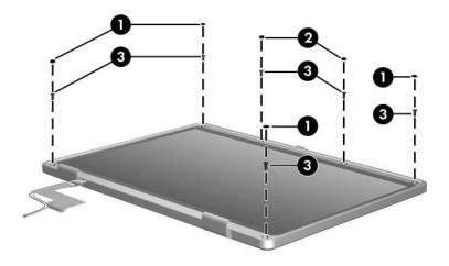
Removing the Display Bezel Screws, Compaq Presario V4000 Models
