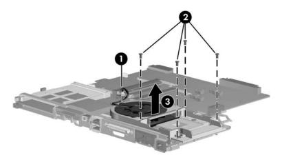
Removing the Fan Assembly
