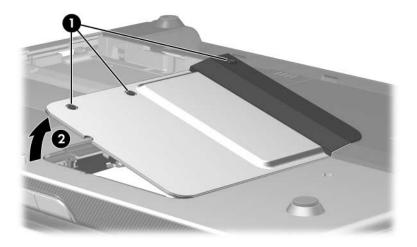
Removing the Memory Module Compartment Cover
