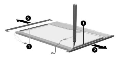
Removing the Display Frame
