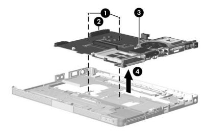
Removing the System Board, Compag Presario V4000 Models
