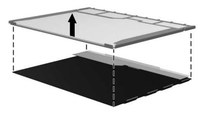
Removing the LCD Panel
