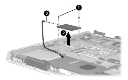
Removing the Modem Board
