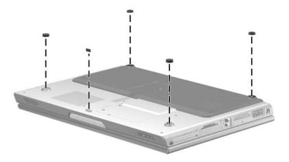
Replacing the Computer Feet, HP Pavilion dv4000
