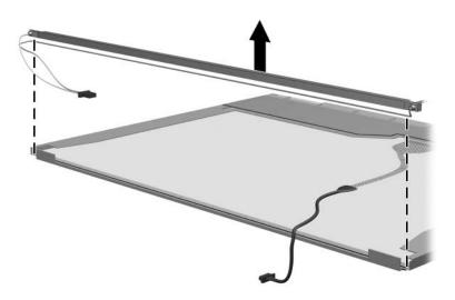
Removing the Backlight Frame
