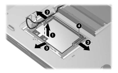
Removing a Mini PCI Communications Module
