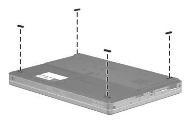
Replacing the Computer Feet, Compaq Presario V4000
