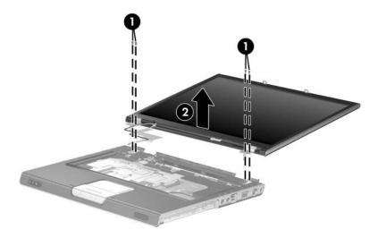
Removing the Display Assembly
