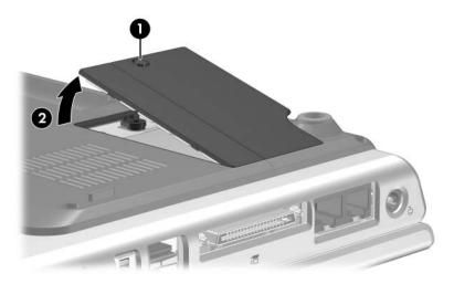
Removing the Thermal Cover
