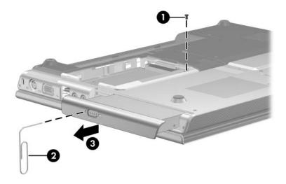
Removing the Optical Drive
