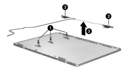
Removing the Wireless Antenna Transceivers and Cables, Compaq Presario V4000 Models
