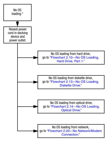
\*NOTE: Before beginning troubleshooting, always check cable connections, cable ends, and drives for bent or damaged pins.
