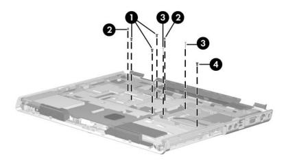
Removing the System Board Screws, HP Pavilion dv4000 Models
