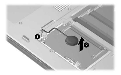
Removing the RTC Battery
