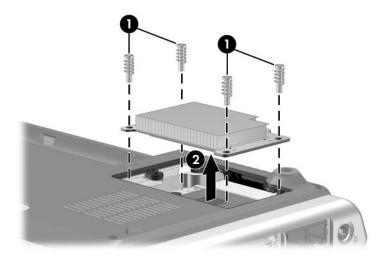
Removing the Heat Sink
