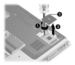
Removing the Processor
