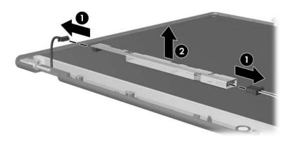
Removing the Display Inverter
