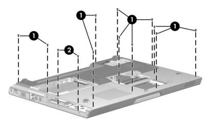
Removing the Top Cover Screws, Part 1, HP Pavilion dv4000 Models
