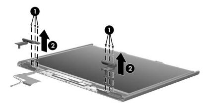
Removing the Display Hinges, HP Pavilion dv4000 Models
