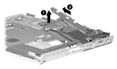
Removing the USB Board and Frame, HP Pavilion dv4000 Models
