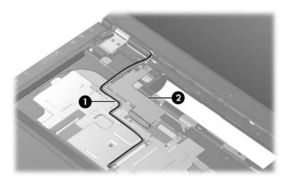
Removing the Wireless Antenna Cables
