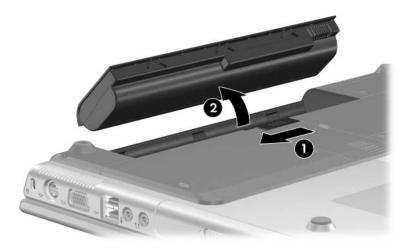
Removing the Battery Pack
