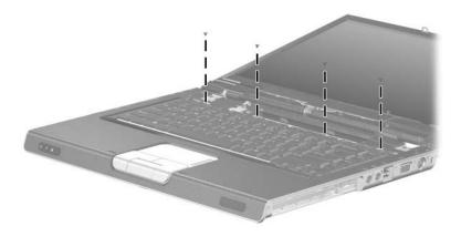
Removing the Keyboard Screws
