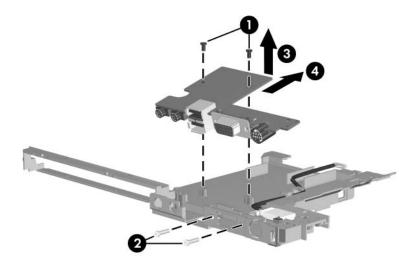
Removing the USB Board
