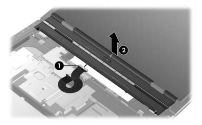
Removing the Switch Cover
