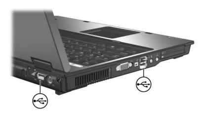
USB hubs can be connected to a USB port on the notebook or on an optional docking device (select models only), or to other USB devices. Hubs support varying numbers of USB devices and are used to increase the number of USB devices in the system. Powered hubs must be connected to external power. Unpowered hubs must be connected either to a USB port on the notebook or to a USB port on a powered hub.
