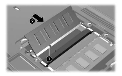
c. Press the memory module downward until the retention clips snap into place.
