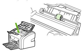
4. Release the small, white tabs on either side of the pickup roller, and rotate the pickup roller toward the front.
